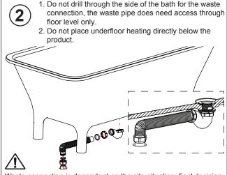
Waste connection is dependent on the site situation; final decision about installation of waste connection should be taken by a suitably qualified person.
